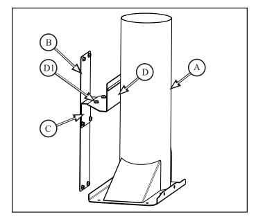
**1.6** Install U-bolt clamp ( $\bf E$ ) around pre-cleaner tube ( $\bf A$ ) and attach to clamp support plate ( $\bf D$ ), with:
